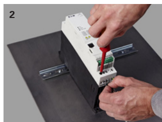
2 Connect mains and motor cables.
